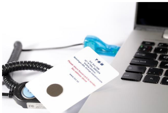
TempTracer data logger connected to computer with T-connector USB
